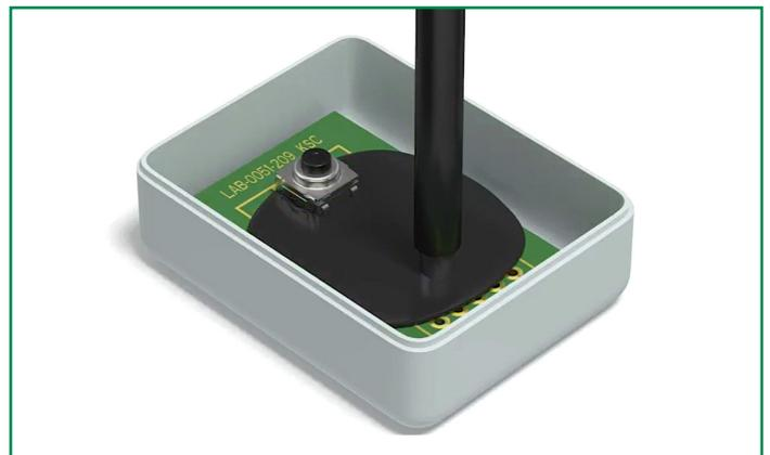
**Figure 1: PCB With a KSCXA Tactile Switch. Process of Being Filled With Potting Material**
