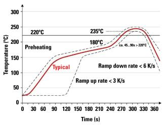
Note: Up to 2 reflow cycles in accordance with the above temperature profile
