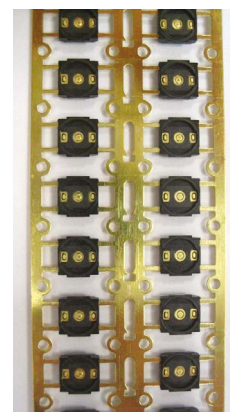
Precision stamping and over molding tools designed and built by C&K
