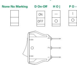
NOTE: Orientation of actuator marking and terminals.
