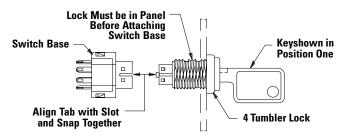
Note: Switch installation is permanent. Switch cannot be removed from lock after assembly. Attempts to separate switch and lock may damage switch.
