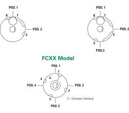
**Notes:** Break-before-make contacts. Terminal numbers are molded on bottom of housing. Actuators are shown in position 1. FAXX models: No common terminal is present. Switching function is provided by movable contacts shorting adjacent pairs of stationary contacts. FCXX models: Common terminal is present. 1. Switches with '02' PC terminations have additional terminal no. 5 as switch support only. This terminal is not connected electrically inside switch.
