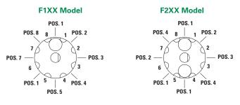
Notes: Break-before-make contacts. Terminal numbers are molded on bottom of housing. Actuators are shown in position 1. FIXX, F2XX models: No common terminal is present. Switching function is provided by movable contacts shorting adjacent pairs of stationary contacts. 1. Switches with '02' PC terminations have additional terminal no. 5 as switch support only. This terminal is
