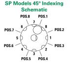
Notes: Break-before-make contacts. Terminal numbers are molded on bottom of housing. Actuators and contacts are shown in position 1
